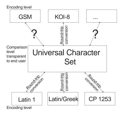
Transparent handling of encoding differences for comparison
